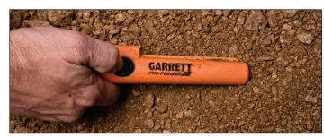
(Above) Fast retune feature quickly tunes out mineralized ground, salt, and other challenging environments.
